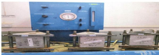
Permeability test apparatus
